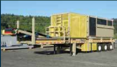
NEW KPI 31 X 44 PIONEER JAW CRUSHING PLANT Vanguard Jaw; Removable Feeder Assembly; Ready to work
