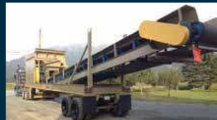
HEAVY DUTY BELT FEEDER 15 yard HD Hopper c/w hyd tip grizzly; 42" Feed Belt - live shaft impact idles; 48" discharge conveyor
