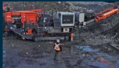
SANDVIK QJ240 TRACK IMPACT CRUSHER Primary & Secondary Impact Crusher; 4 bar rotor 39" wide; 350 HP Cat Engine; Pan Feeder, Pre-Screen
