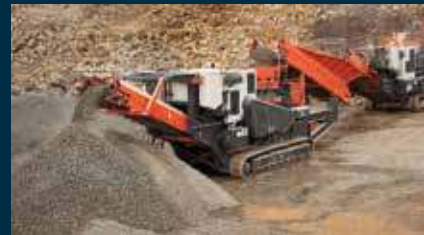
SANDVIK TRACK CONE CRUSHER Sandvik QH430 Cone; 350 HP Cat Engine; 6.5 yard Hopper
