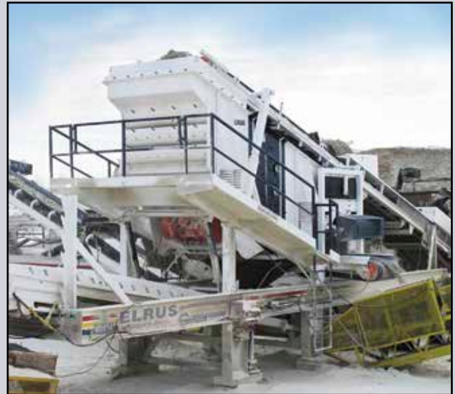
High Capacity 6'x12' 3 Deck Multi-Slope Screen Plant. (More production than a 6'x20')
