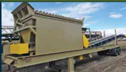
BELT FEEDER 42' with live shaft idlers x 48" discharge, cantilever style grizzly. CALL
