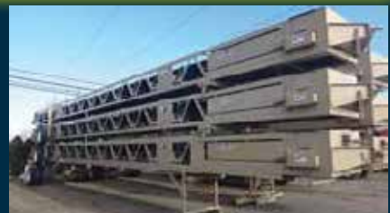
KPI 36" x 60" ROLL PACK CONVEYORS c/w CEIMA "C" idlers, 3 ply belt, belt scrapers. CALL
