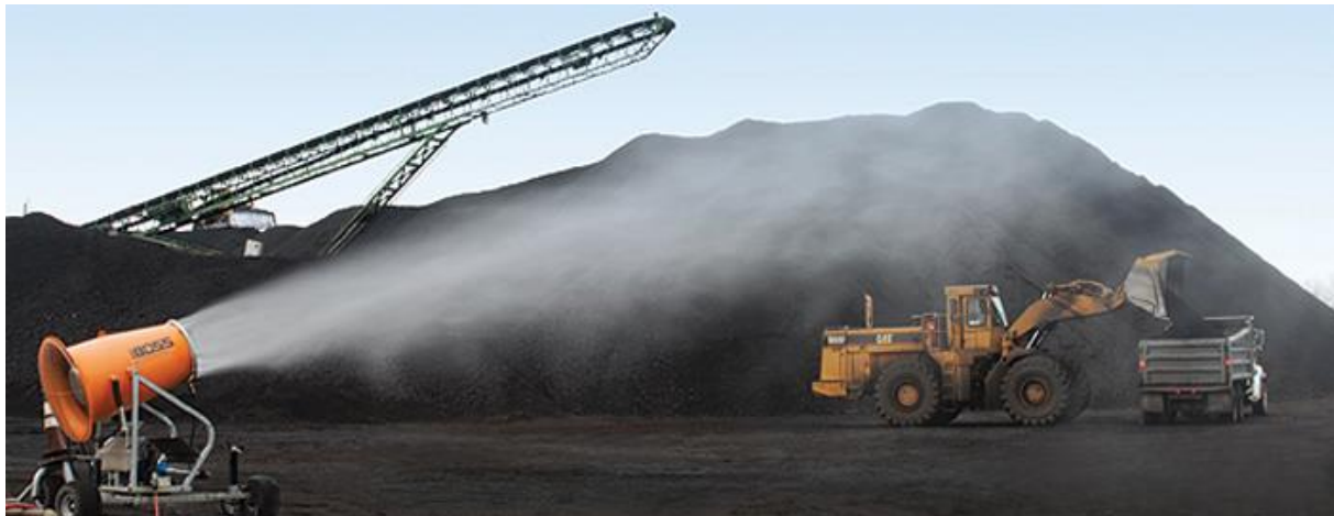
Dust suppression with water spray
